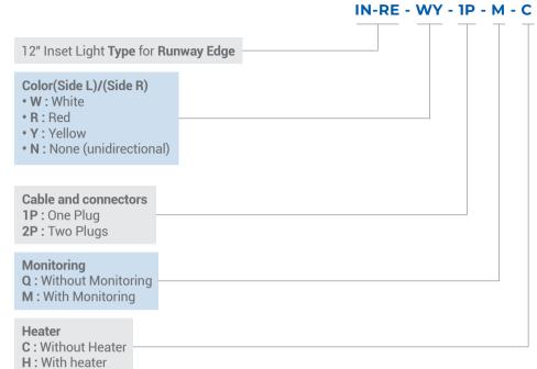
\* The beam aiming is not field adjustable
