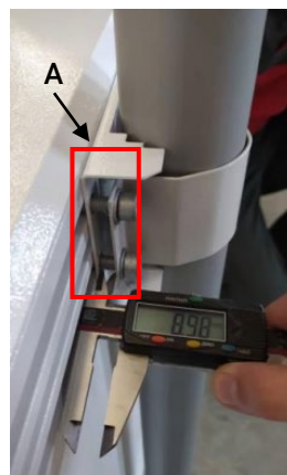
Figure 4-13 Details of the Pole and Pole Holder
