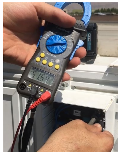
Figure 6-11 Check the output voltage and voltage across the link terminal
